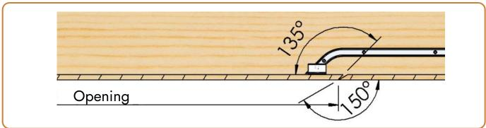
The width of the opening into which the sliding panel enters can be up to 3000 mm.
