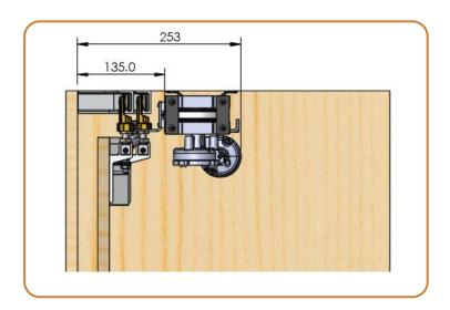
The connecting rod is as parallel as possible to the door panel, although this is not critical. Logically, the module 'pulls' the door open and 'pushes' it closed. The distance H is the horizontal position of the connecting corner piece and is determined when the door is closed and the carriage of the module is in the forward position.
