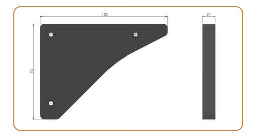
The guide plate is placed on the bottom against the side of the cabinet 40 mm from the front.
